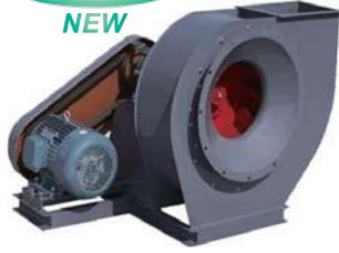
The 4-72(C) type backward curved centrifugal ventilator is widely used for the ventilation & smoke extraction in the kitchen of canteens, restaurants & hotels. Also, it is widely applicable for the agricultural, chemi-industrial, plastic industrial machines & equipments. The air or gas that is being delivered by the fan should be  $\leq 80^{\circ}\text{C}$ , and without any gunk, dust or rigid granule of no bigger than  $150\text{mg}/\text{m}^3$ .
